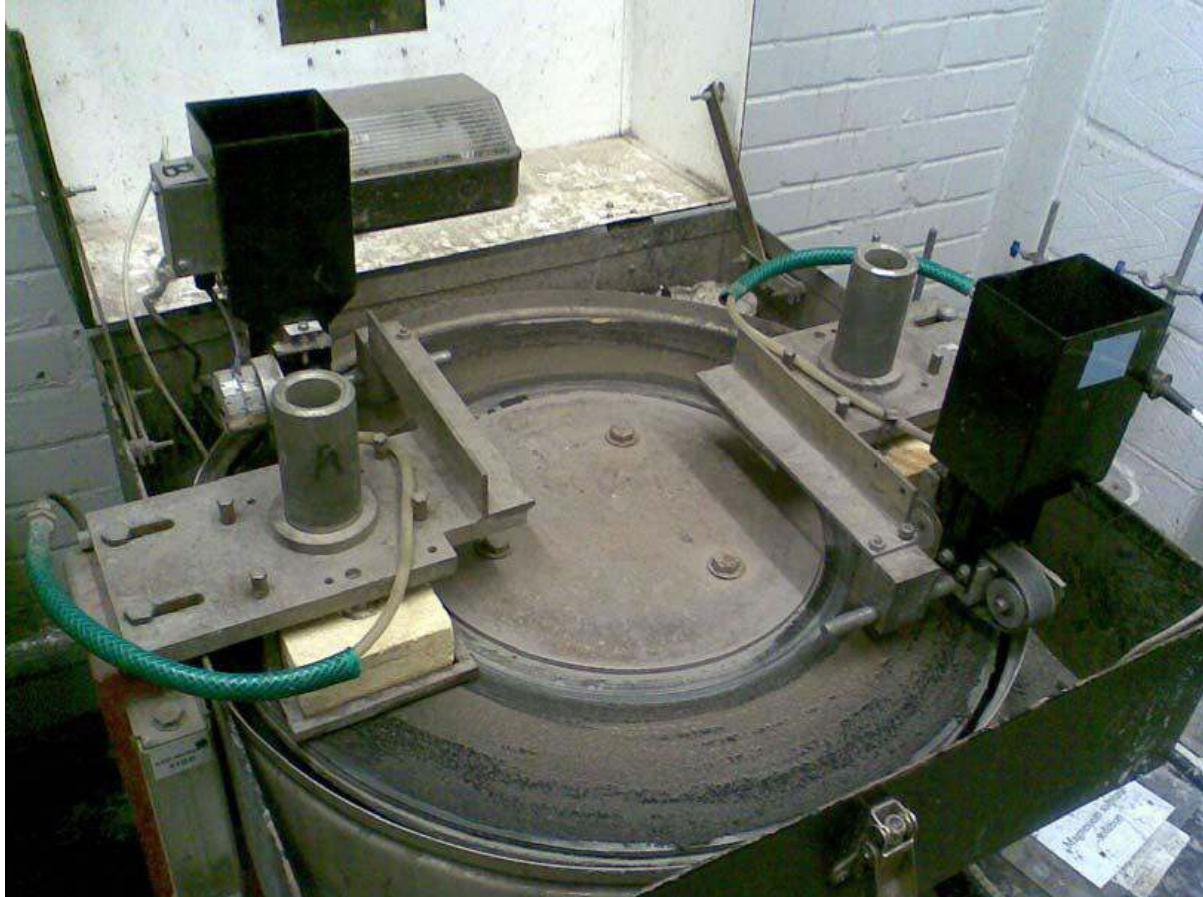
Figure 1 The accelerated polishing machine
