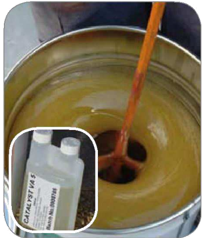
Mixing the base component with a paddle
