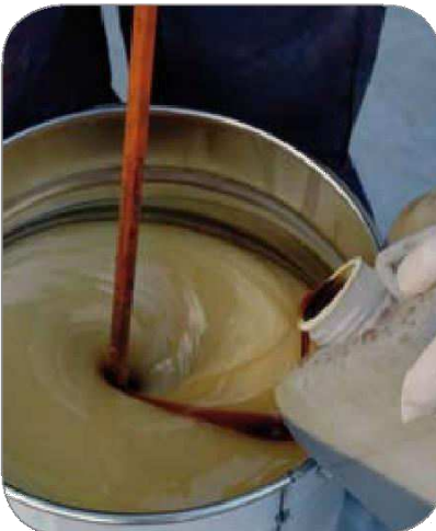
Add the activator slowly whilst mixing
