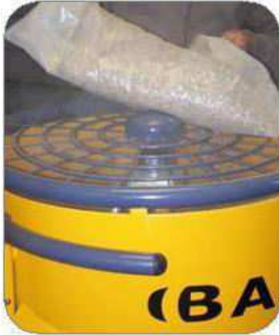
Charge the mixer with aggregate
